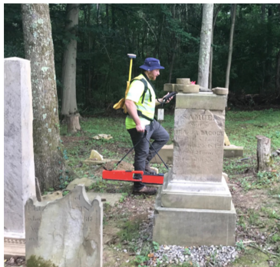
Using electromagnetic induction methods to map grave locations at an abandoned cemetery, Pennsylvania.
