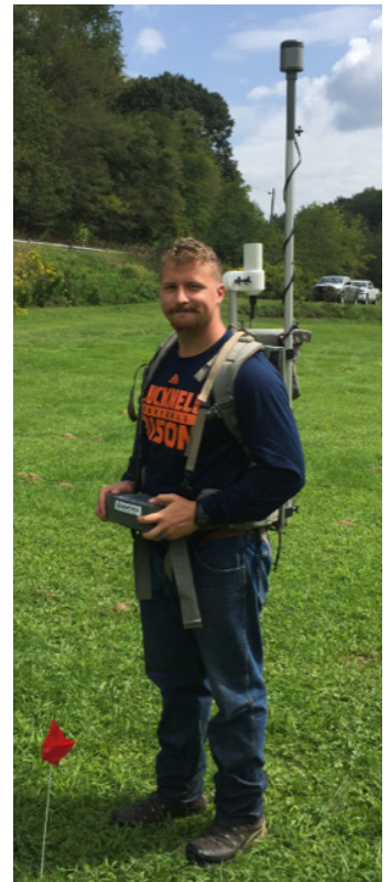
Magnetometer and GPS configuration for detailed mapping of abandoned gas wells, Appalachian Basin.
