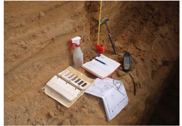
A thorough soils investigation uses the right tools for the job including a Munsell color chart, spray bottle and a gps receiver; used here to describe soil developed in loess overlying fluvial deposits.
